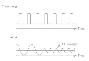
When the air leakage reaches 60lpm, it can still be triggered synchronously.
